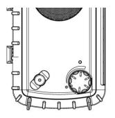
Power LED: The LED above the volume knob is 'on' when the batteries are in use even if you do not hear sound from the speaker. To optimize the lifespan of the batteries please turn the Eco Extreme off when not listening to music.
